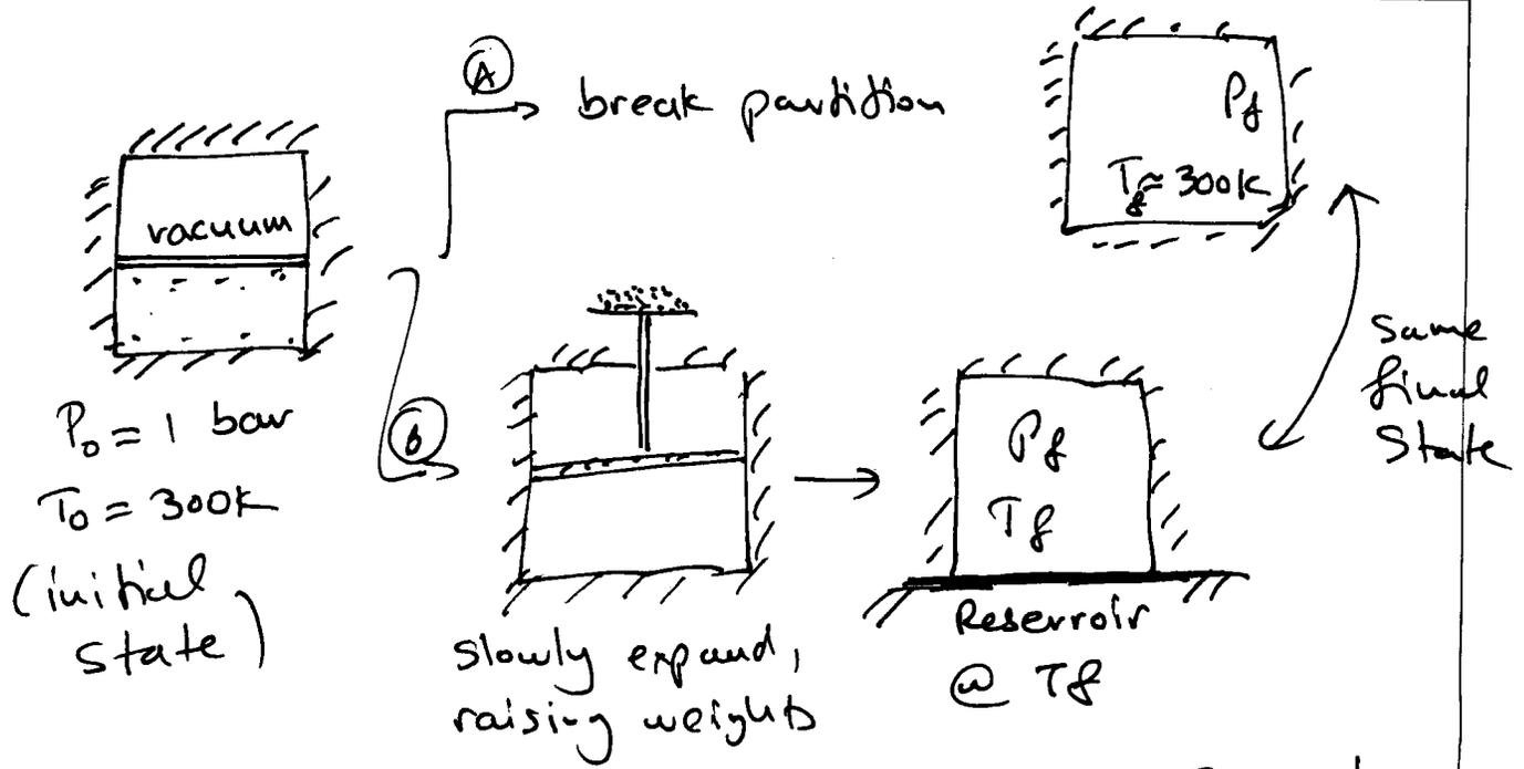
$$\underbrace{\Delta E}_{\text{Change in Energy of gas}} = \underbrace{Q}_{\text{heat input}} + \underbrace{W}_{\text{work input}} \quad \parallel \text{ First Law Closed Systems}$$
